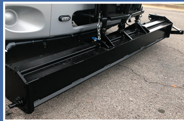
POWERFUL MAGNET TO COLLECT FERROUS MATERIAL
