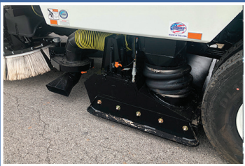
VACUUM AND BRUSH REMOVAL OF DEBRIS
