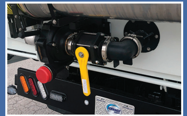
GLYCOL RECOVERY FOR PICKING UP DE-ICING FLUID
