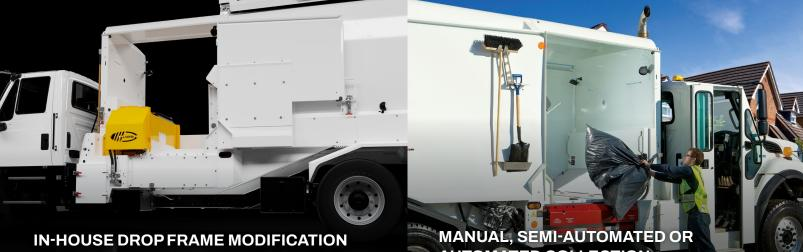
Labrie<sup>™</sup> is the only manufacturer that conducts the drop frame modification process in-house. This gives us direct control over the process, ultimately benefiting our clients.
