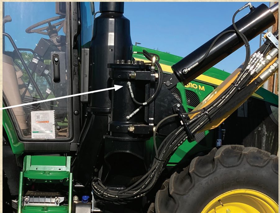
CLOSE UP OF HYDRAULIC ACTUATOR
