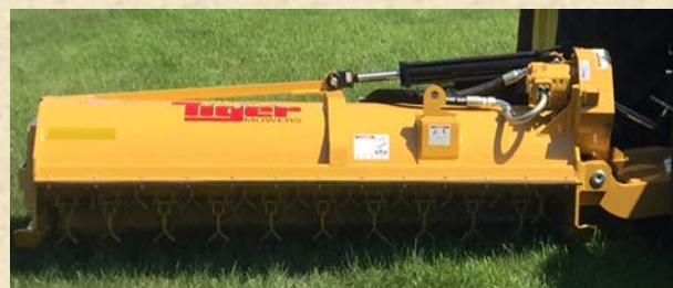
75" side flail with standard cut knives Available in 60", 75" and 90" sizes
